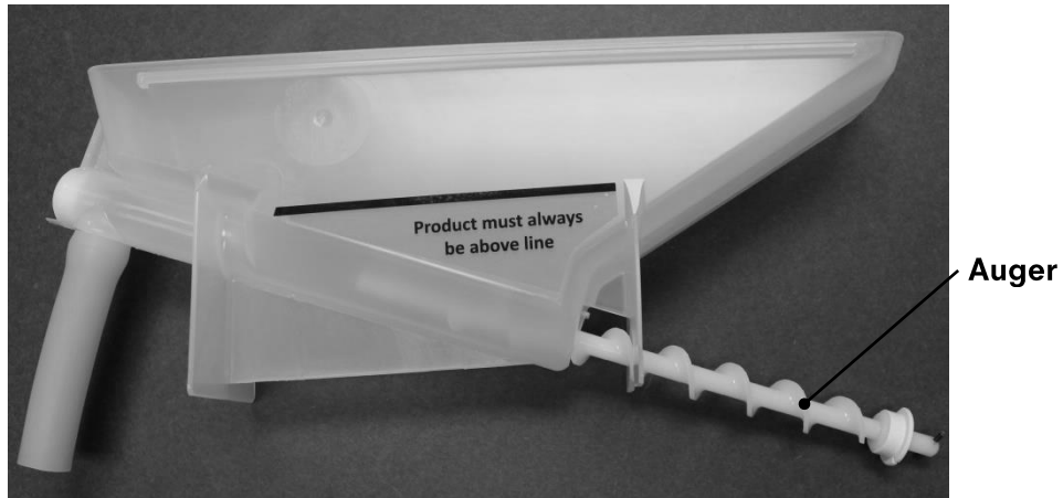
Figure 15: Remove auger from back of hopper
